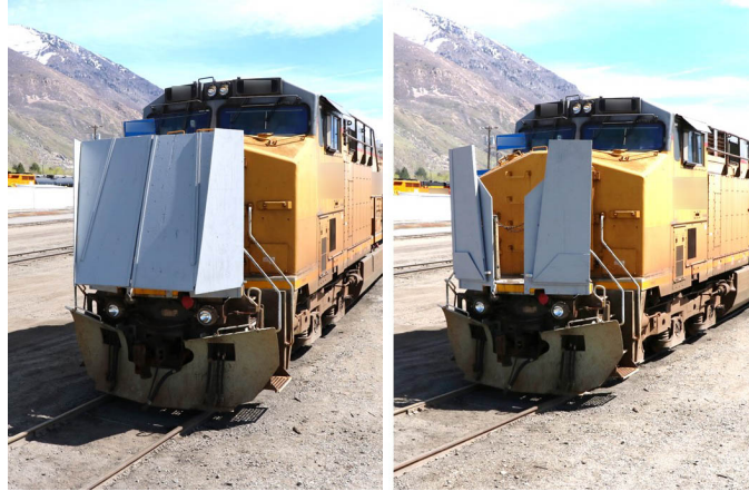
Figure 2: Full-scale prototype of the origami-inspired deployable fairing on a freight locomotive shown in both the deployed configuration (left) and stowed configuration (right). Photo has been modified to remove locomotive identity.
